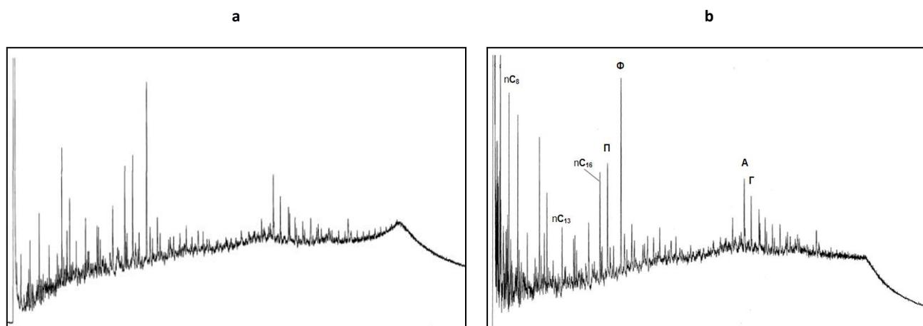
**Figure 3: Chromatograms of the transformed naphtha: a) naphtha initial; b) naphtha, hexane, Co[acac]<sub>3</sub>**
